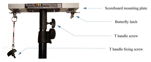
Ensure that the two butterfly latches hang down and out of the way. Lift the scoreboard onto the mounting plate, aligning the edge of the mounting plate with the two alignment arrows on the front of the scoreboard. Hold the scoreboard in position while attaching it to the mounting plate using the two butterfly latches.
